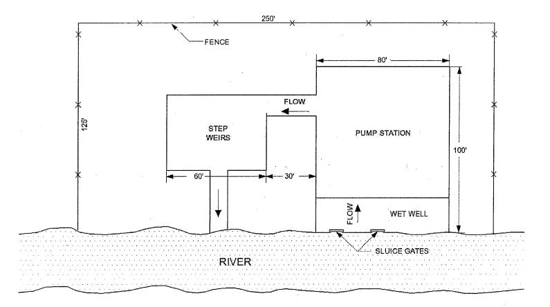
Figure 4.11 – 80 g/s (Oxygen) SEPA Station Conceptual Layout
