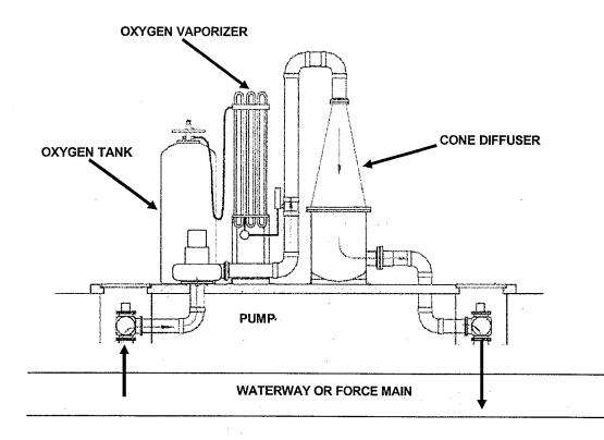
Figure 4.9 – Schematic of Pressurized HPO Contactor
