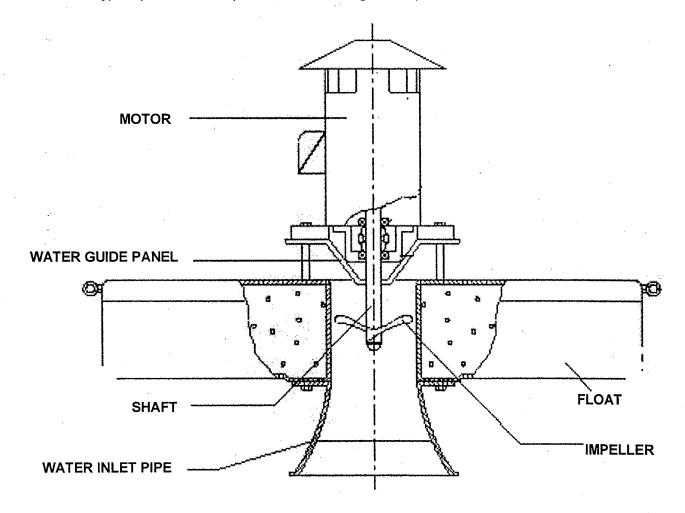
Figure 4.7 - Mechanical Surface Aerator
