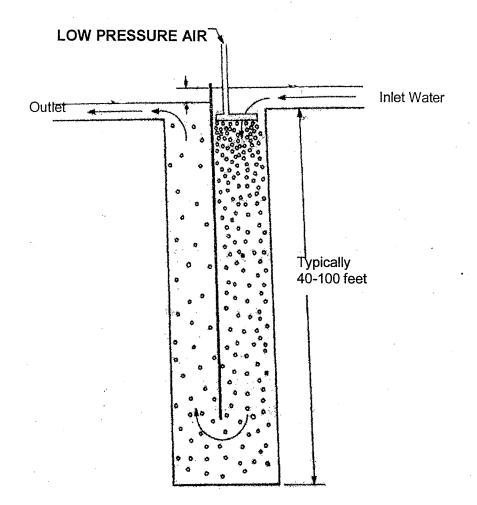
Figure 4.8 – Schematic of Compressed Air U-Tube Contactor
