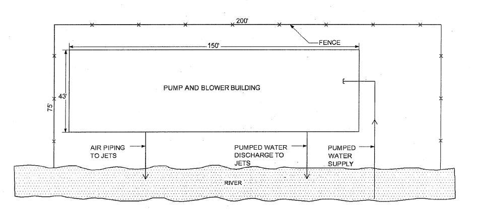
Figure 4.12 – 80 g/s (Oxygen) Jet Aeration Station Conceptual Layout
